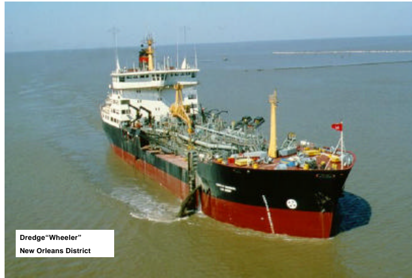
Figure 6-6. Typical USCG Maritime DGPS controlled Corps hopper dredge at Southwest Pass, LA (New Orleans District)
