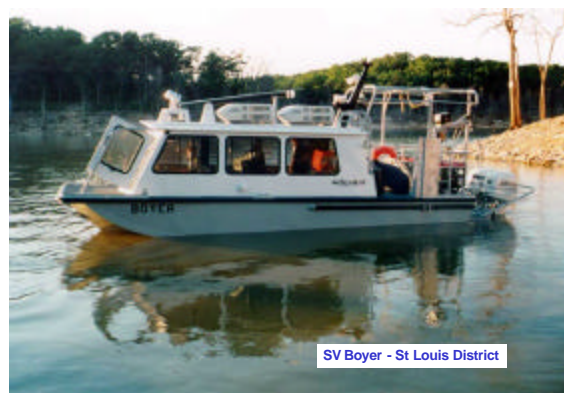
Figure 6-9. St. Louis District hydraulics and hydrology survey boat
